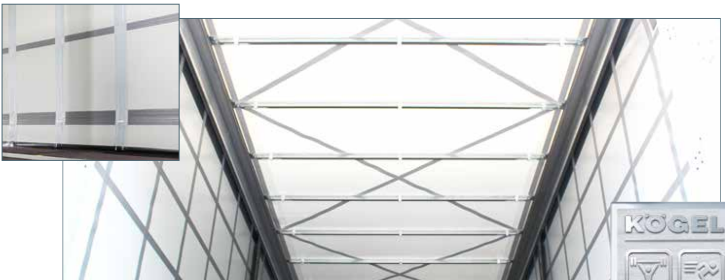
Single-level and twin-level beverage transport possible without lattices thanks to integrated restraint system in the tarpaulin.
